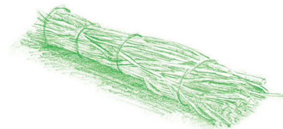
Figure 18: Bundles of branches (fascines) as alternative to wooden logs
