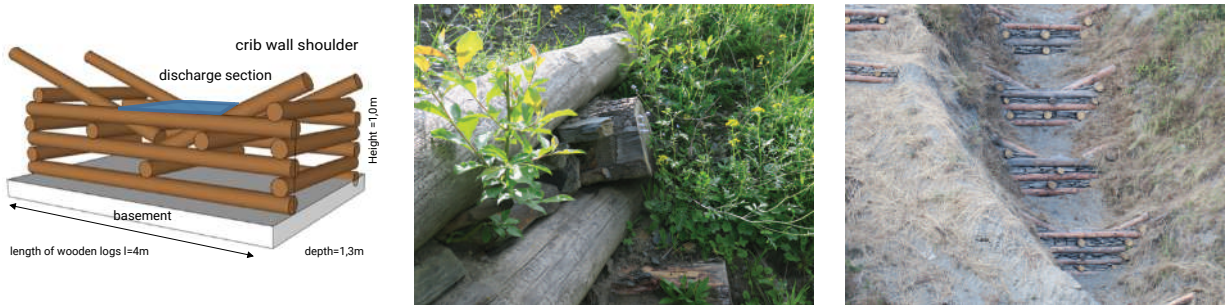
Figure 36: Vegetated wooden check dams
